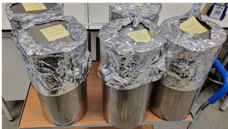
Figure 1. Part 2 – Sample containers for measurements of release of chemical additives from plastic consumer products to surfaces.
