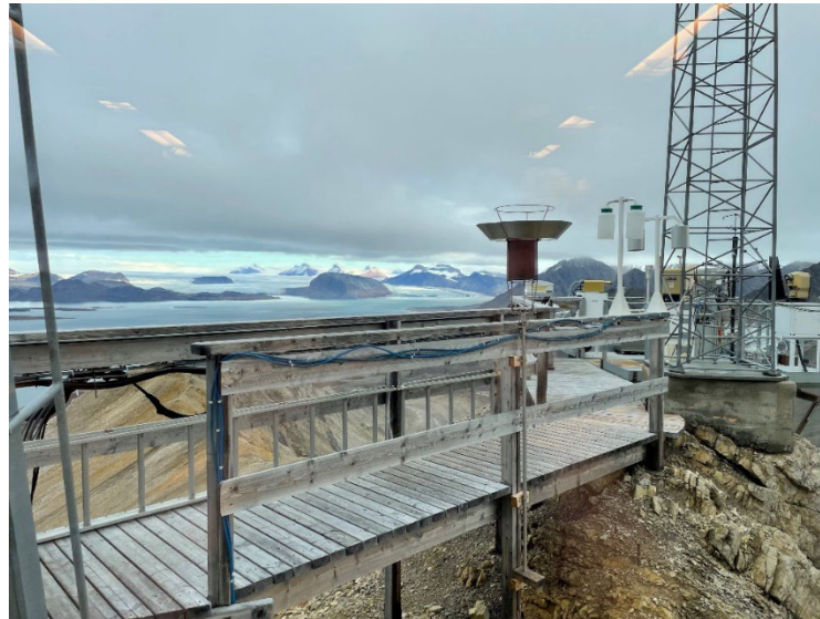
Figure 39. Illustration of deposition sampler at Zeppelin station, photo by Dorte Herzke.
